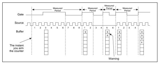
Figure 2-26. Buffered Period Measurement when No Source Edges Are Present between Gate Edges
